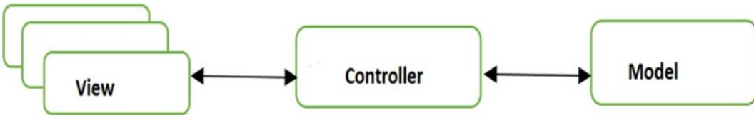
Figure 26-3. An MVC framework with multiple views
