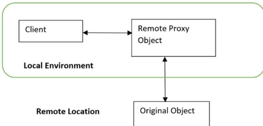
**Figure 6-3.** A simple remote proxy diagram
