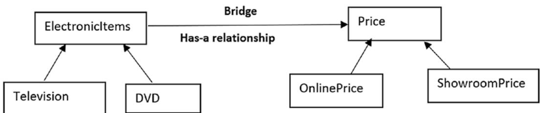
**Figure 12-3.** Maintaining two separate hierarchies using the Bridge pattern
