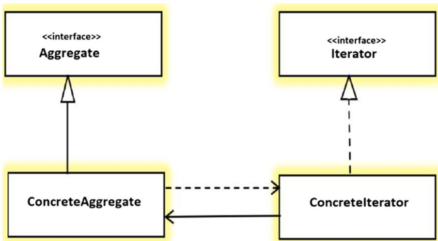
**Figure 18-1.** A sample diagram for an Iterator pattern
