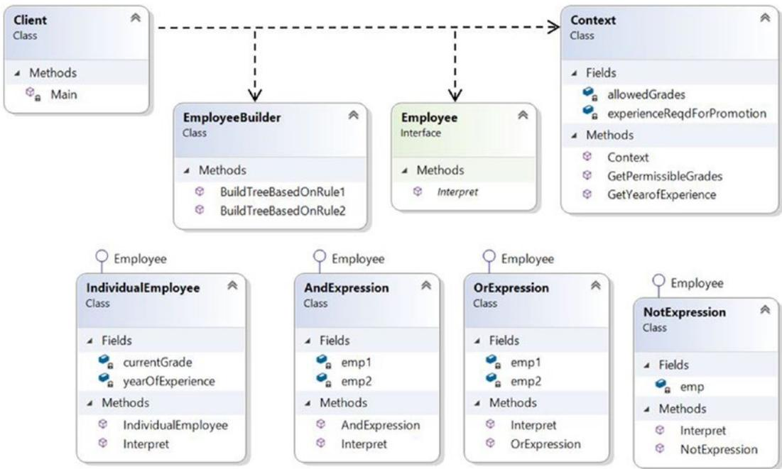
Figure 23-4. Class diagram
