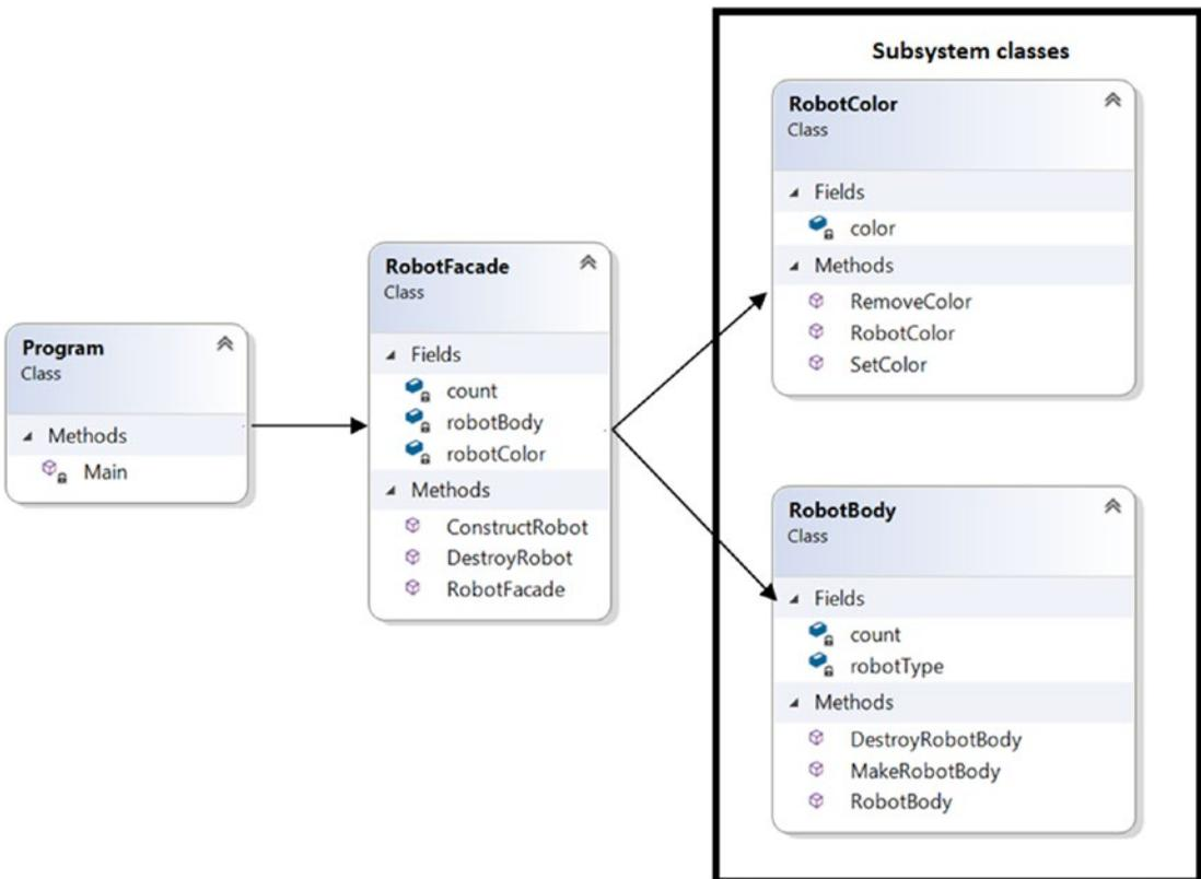
**Figure 9-1.** Class diagram
