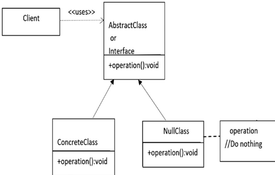
**Figure 25-1.** The basic structure of a Null Object pattern
