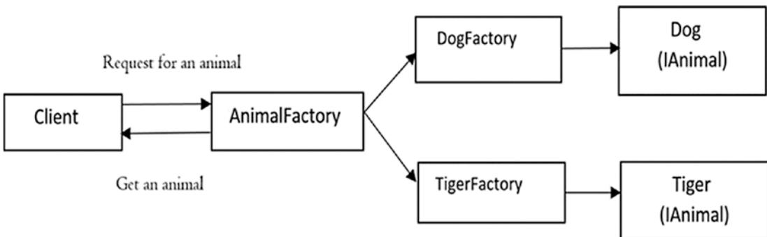
**Figure 5-5.** Factory Method pattern
