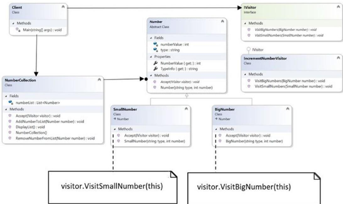
Figure 13-1. Class diagram
