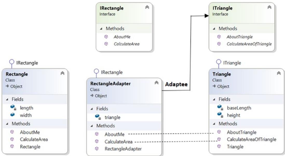
**Figure 8-4.** Class diagram. Client class is not shown here.
