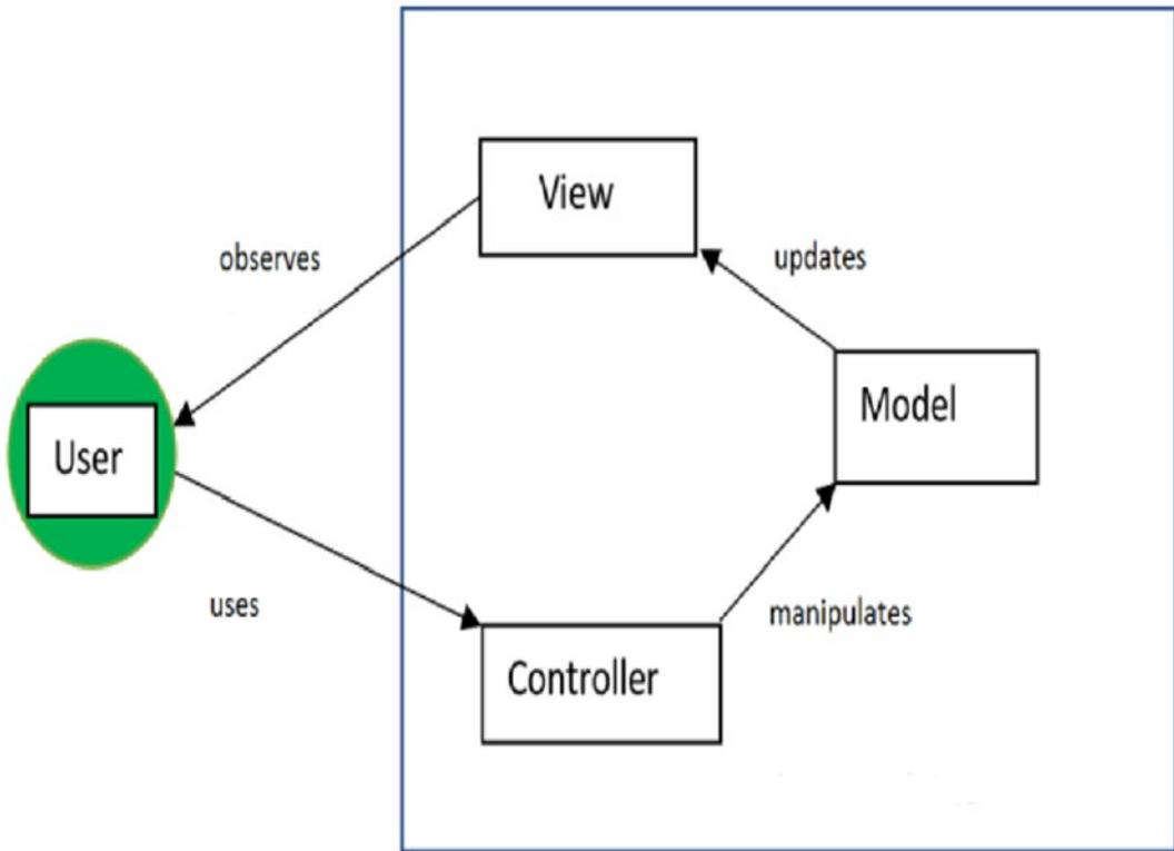
Figure 26-2. A typical MVC framework
