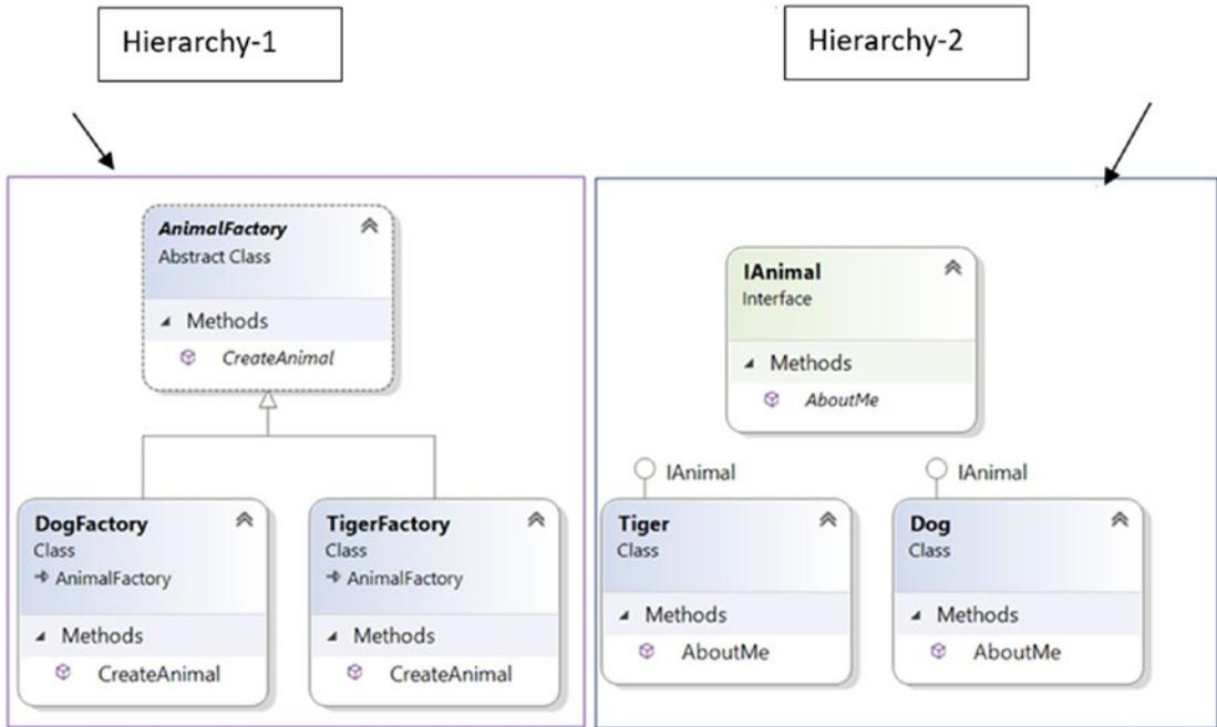
**Figure 4-3.** The two class hierarchies in this example
