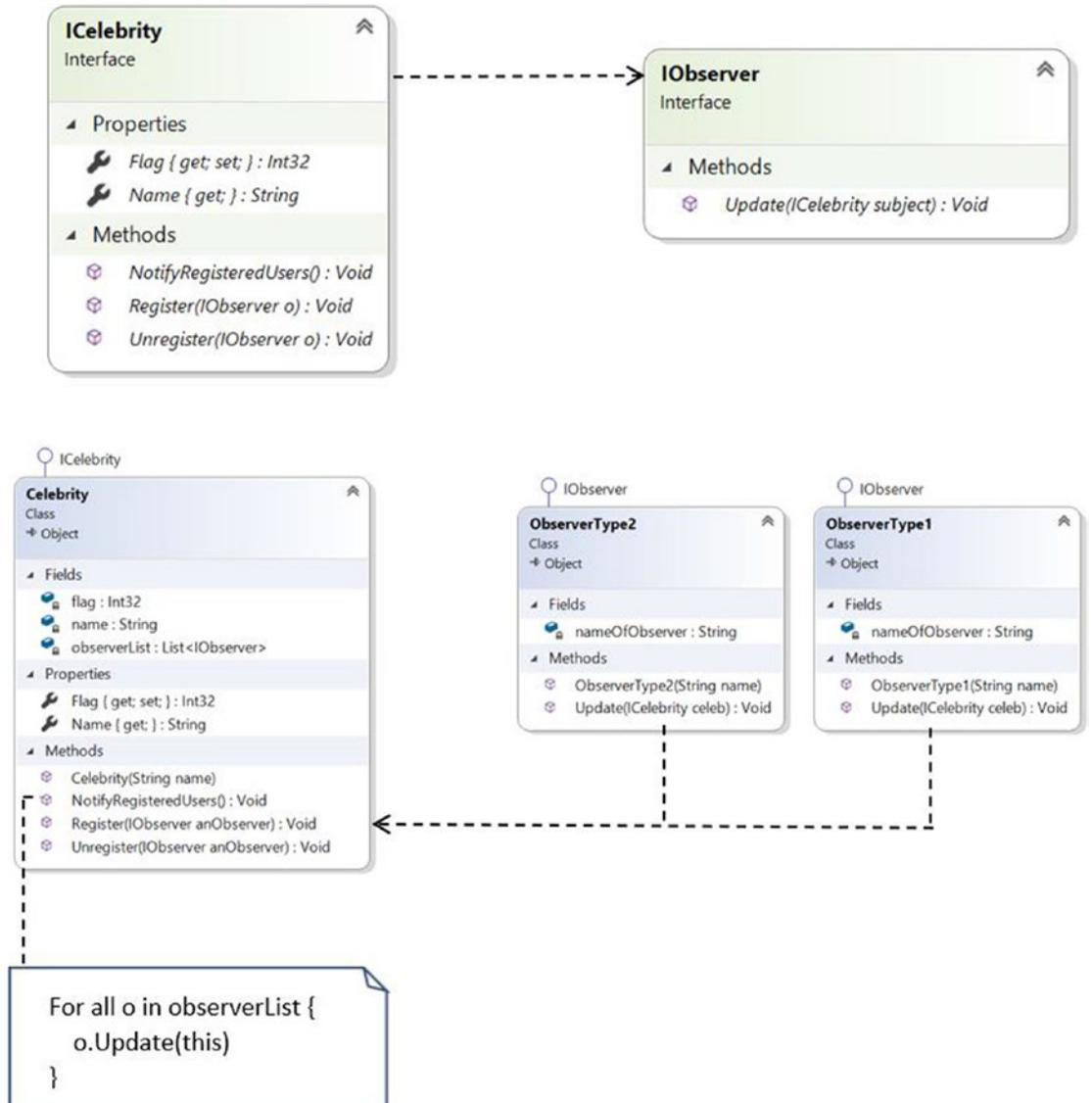
Figure 14-6. The class diagram
